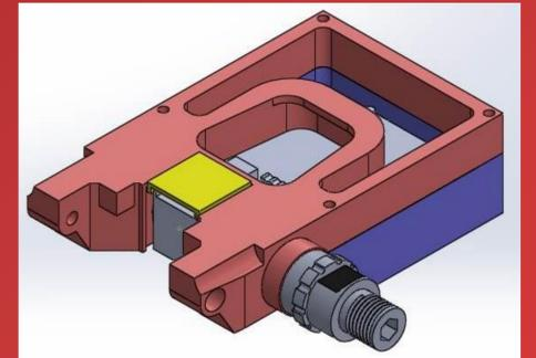
After completing the final CAD design, our group had the pedal 3D printed to ensure correct dimensions and fit. The pedal fits onto the bike by screwing it onto the spindle (seen below, left) and allows for the shoe to be clipped into it (seen below, right). The electronic components all fit in the bottom half of the pedal (seen below, middle), safely away from the shoe cleat. The top and bottom halves are secured with 4 screws which allows for easy maintenance and repair.
