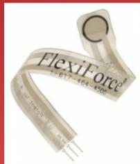
The design makes use of many components to meet these specifications. The Flexiforce sensor (seen left) measures the force on the pedal. An Arduino microcontroller (seen right) receives force data and computes the rider's power output. The power is transmitted via Bluetooth Mate to a SmartPhone app.
