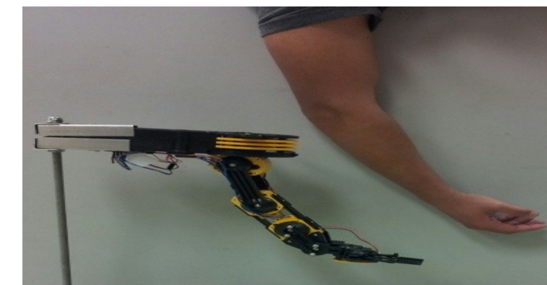
Fig. 2 Robotic Arm Stand simulating human arm
