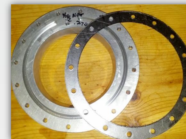
Figure 3: High-temperature Graphoil seals
