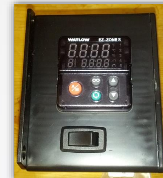
Figure 4: PID controller for heating coil.
