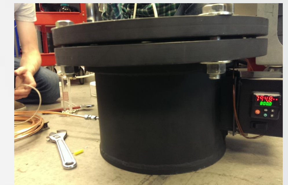
Figure 10: Empirical test with flow rates of 2 L/min – 4 L/min taking various temperature reading along copper tube. Validated flow simulation
