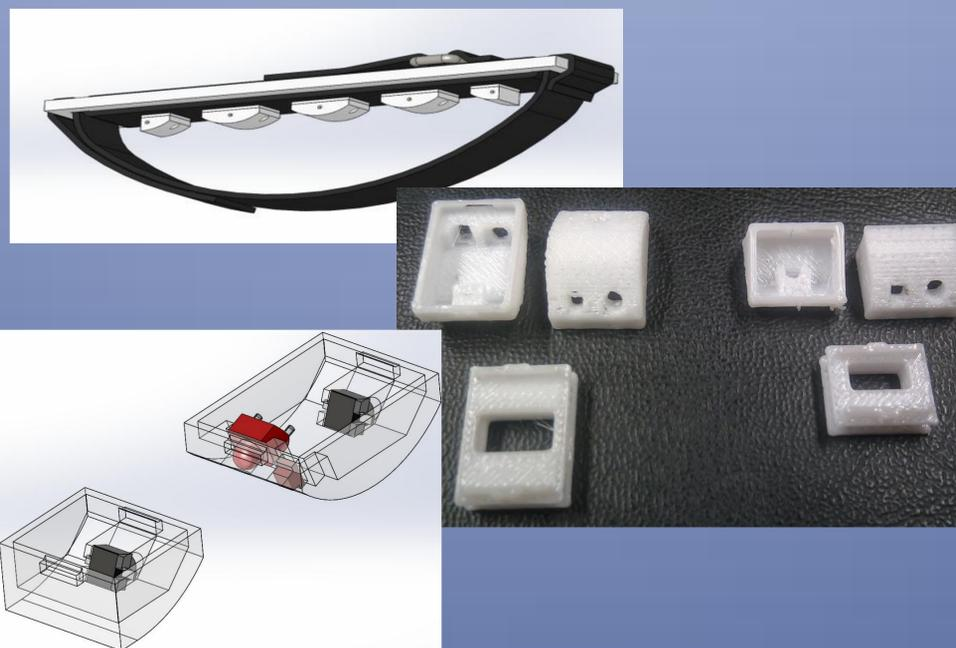
The sensors are placed into a semi-circular housing which fit comfortable between the users knuckles in order to ensure the closest possible sensor readings and minimizing noise as much as possible.
