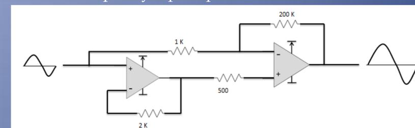
Our final amplifier circuit (above) made use of the MCP6004 microchips. A gain of ~100 was necessary to extract the desired signal.
