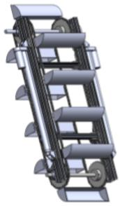
**Tilting deposition bin with** a tensioned gate: In-house welded aluminum bin that tilts to deposit regolith. A tensioned gate automatically opens when tilted & closes when leveled.
