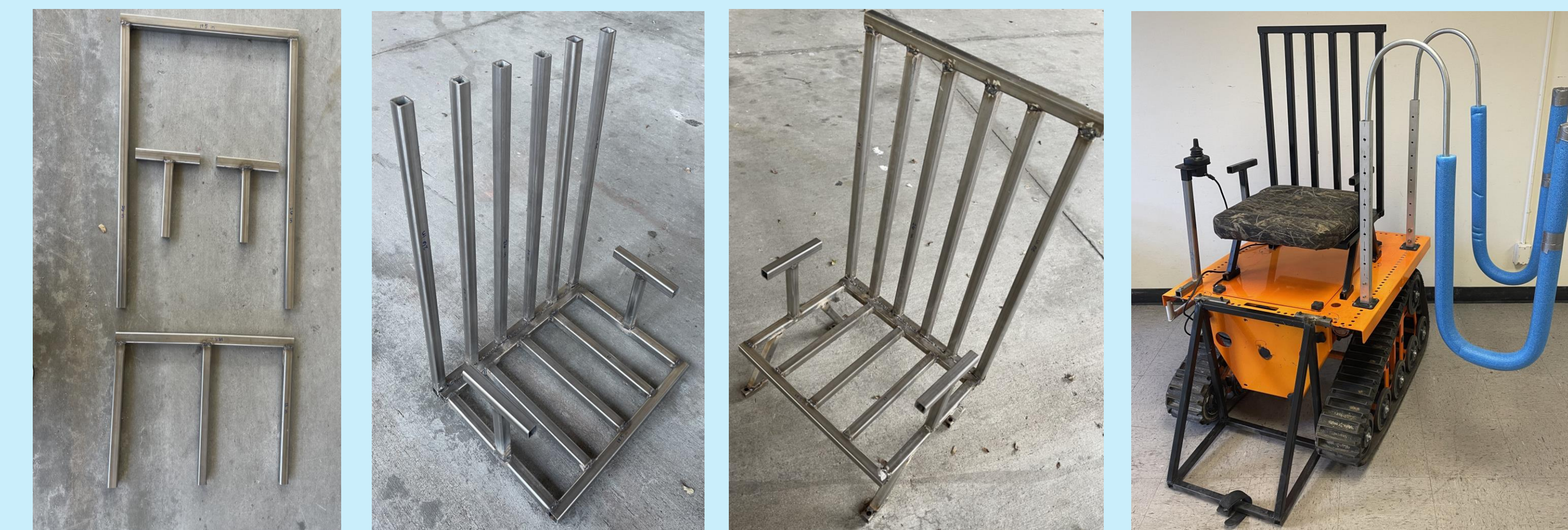
Flux Core Welding performed to construct chair and leg rest
