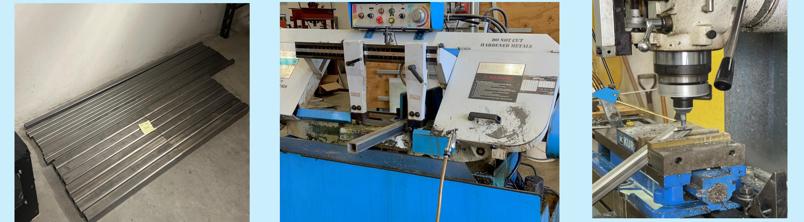
Band Saw, Cold saw and CNC Mill used to prep steel bars for welding
