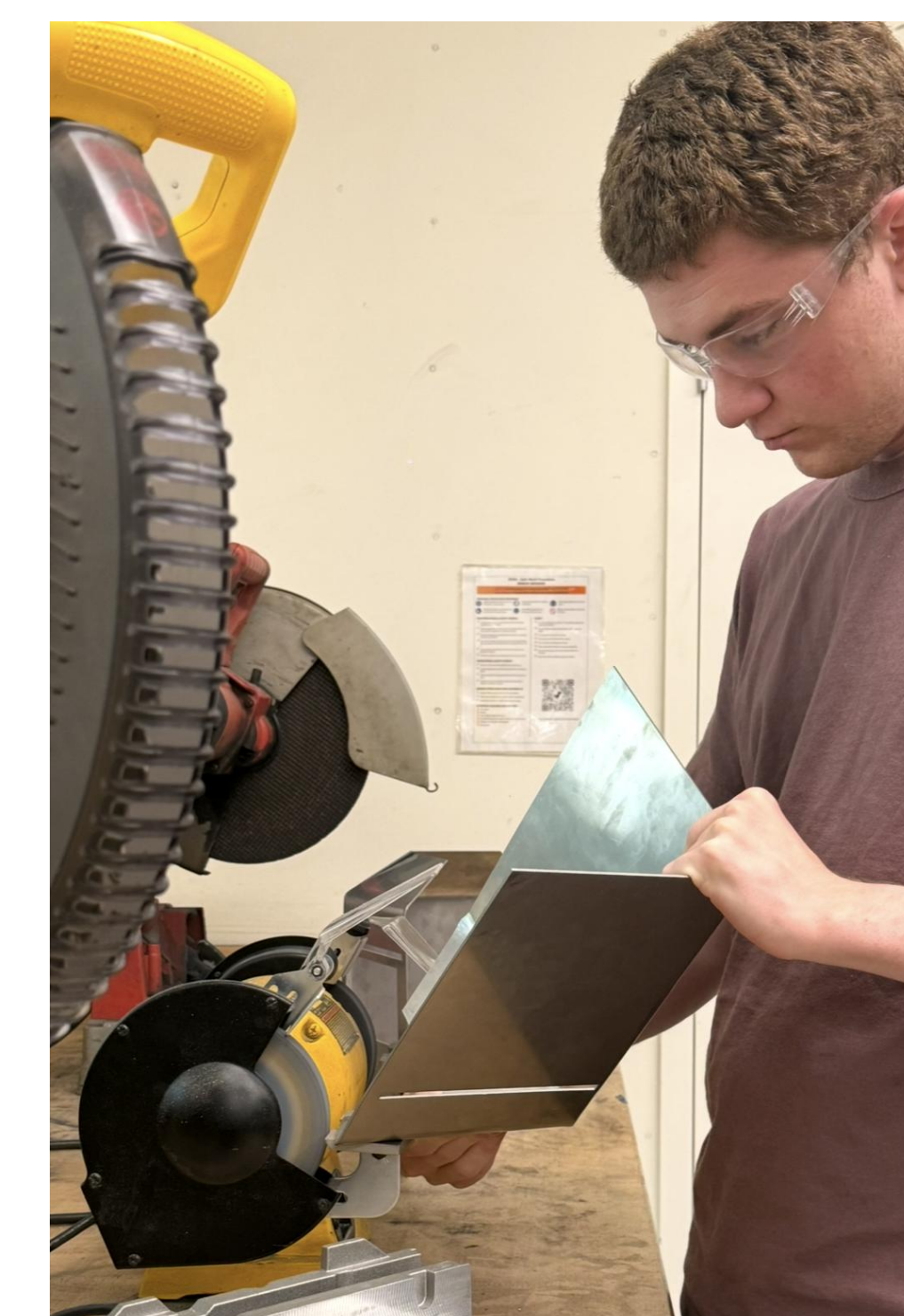
Grinding Combustion Chamber Edges for Welding
