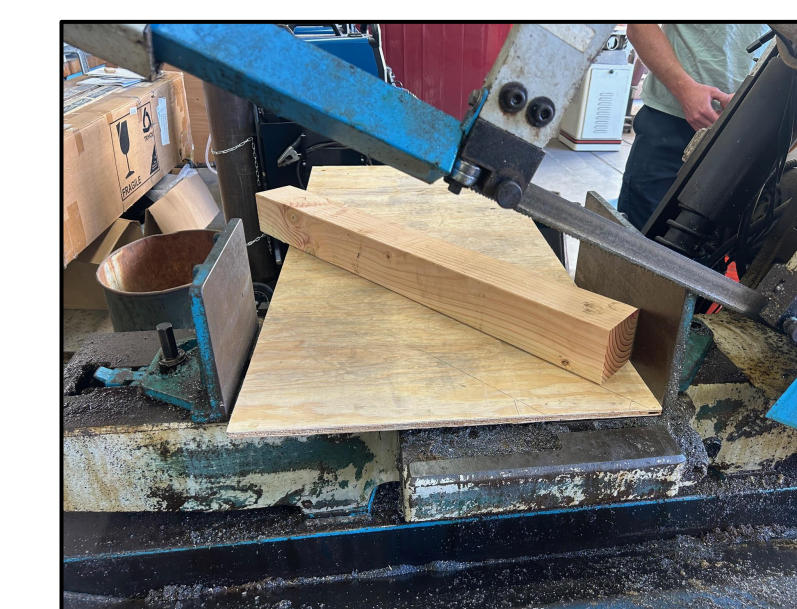
Final Assembly of Jig for Angled Cuts
