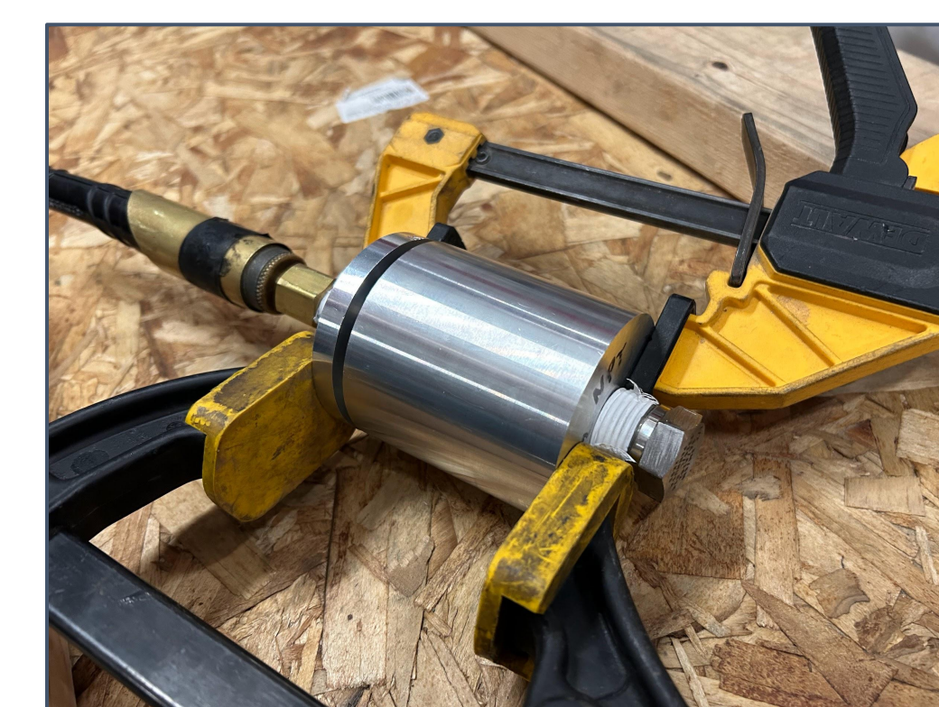
Pressure Testing of Seal Component
