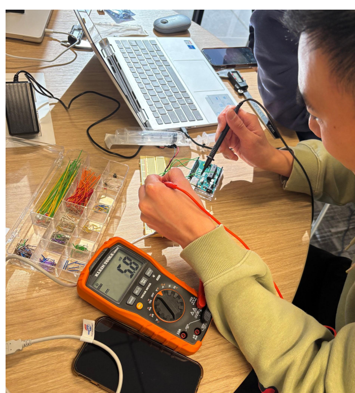
Measuring the voltage of the Arduino pins to troubleshoot the circuit
