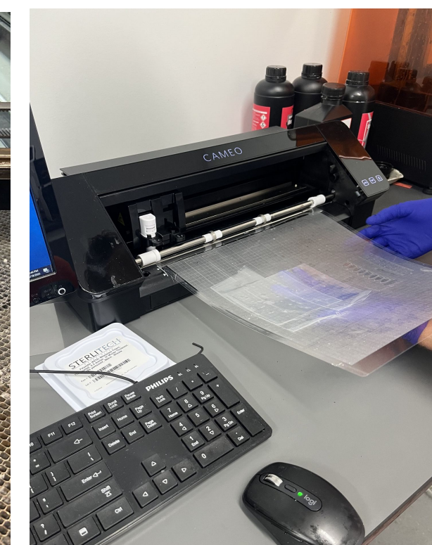
Craft cutter used to create the valves instead
