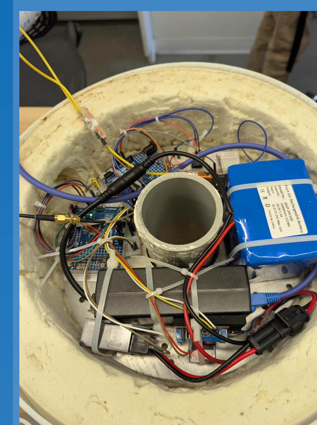
The lower half of the buoy, housing the electronics payload.
