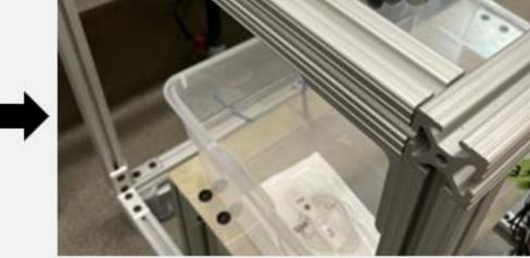
The filled pouch is dropped below into a bin.
