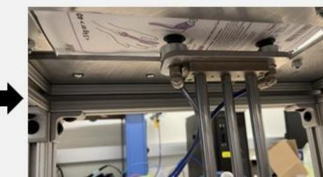
The linear actuator extends to suction on to pouch.
