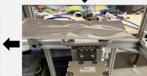
The linear actuator retracts to remove pouch from the hopper.
