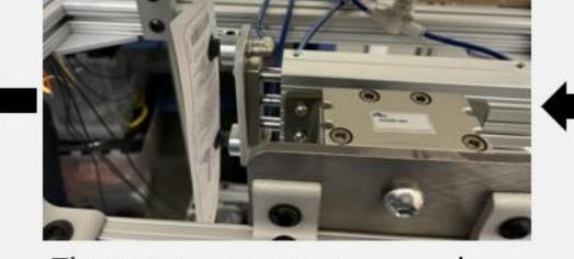
The rotary actuator rotates the linear actuator assembly 90°.
