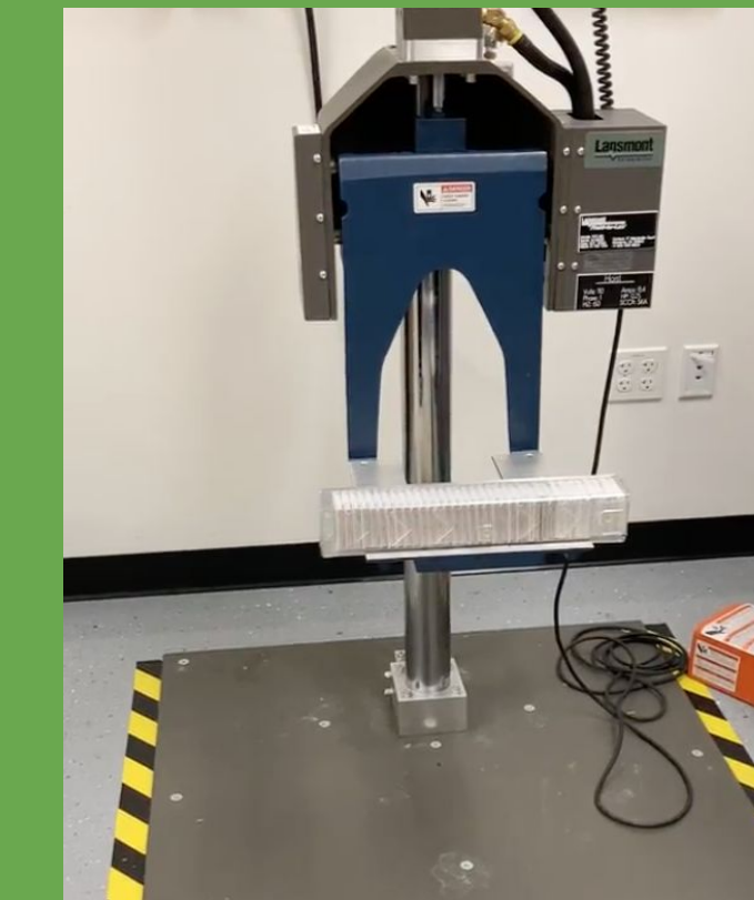
Square tray tested on the Drop Tester
