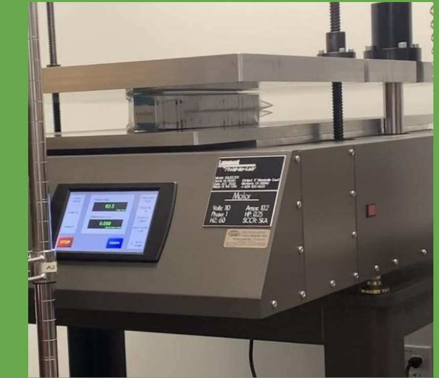
Triangle tray tested on the Lansmont Compressor
