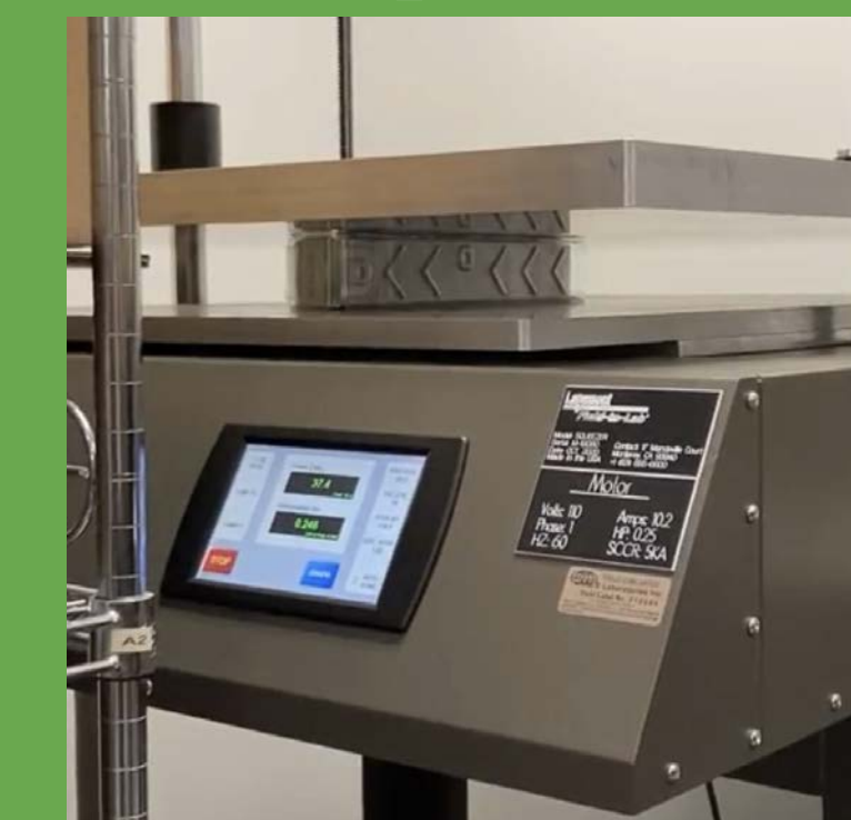
Square tray tested on the Compressor
