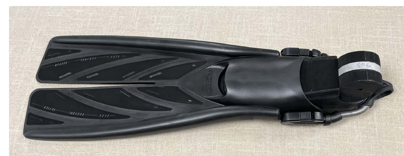
Foot and Fin prototype (1:1 scale); our foot CAD model was 3D printed to test fit it in a standard SCUBA fin before it was casted out of silicone.
