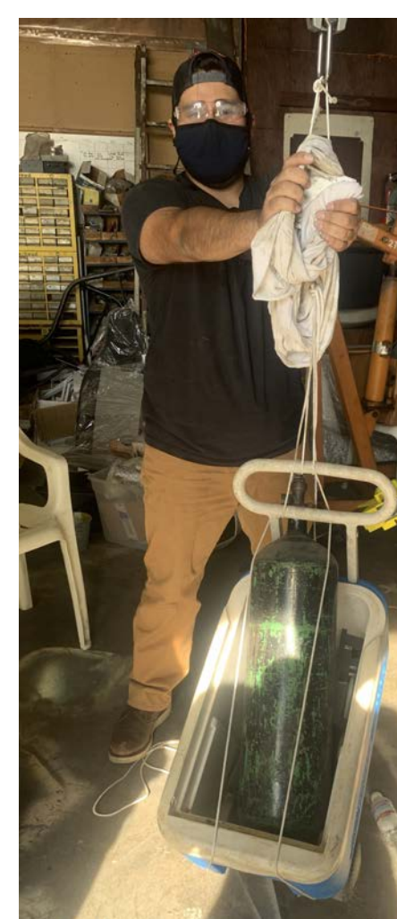
A load test was conducted at Gillespie Field to verify that our epoxy selection can support a maximum shear load of 150lbf.
