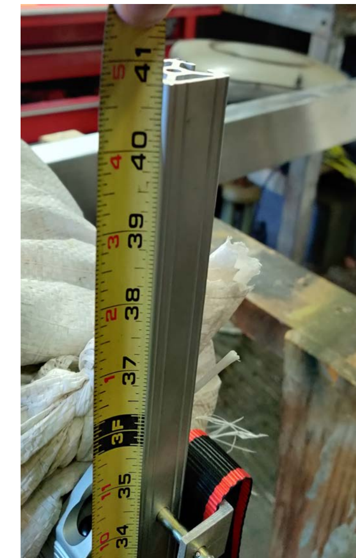
A load test was conducted on our auxiliary mount to determine how far the aluminum extrusions deflect under extreme flight conditions.
