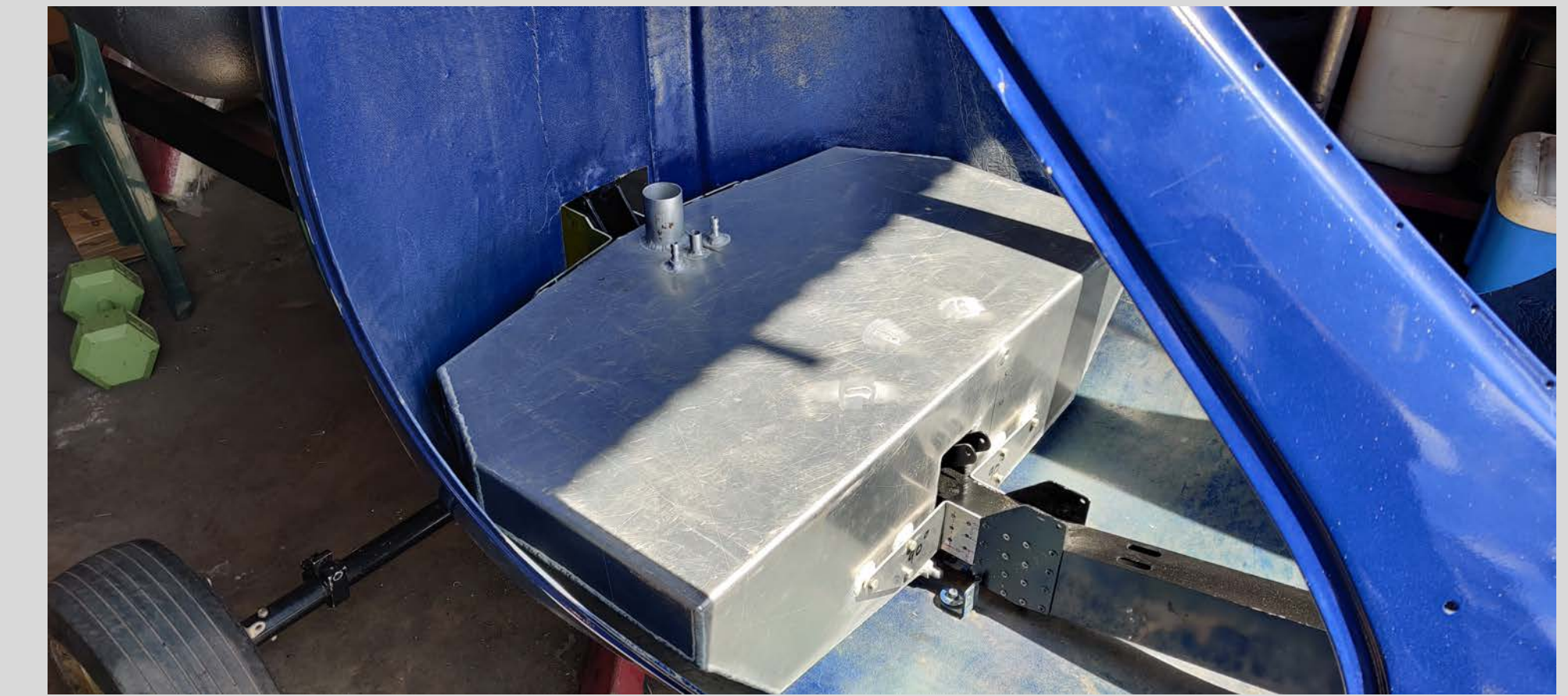
Isometric view of the installed main tank.
