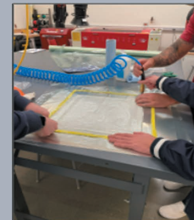
6. Vacuuming Excess Resin
