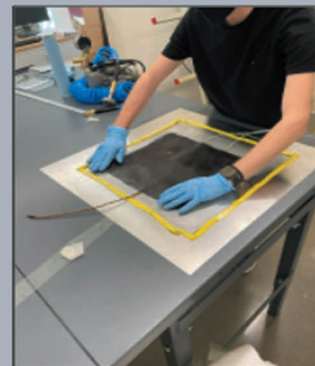
4. Final Carbon Fiber Layers
