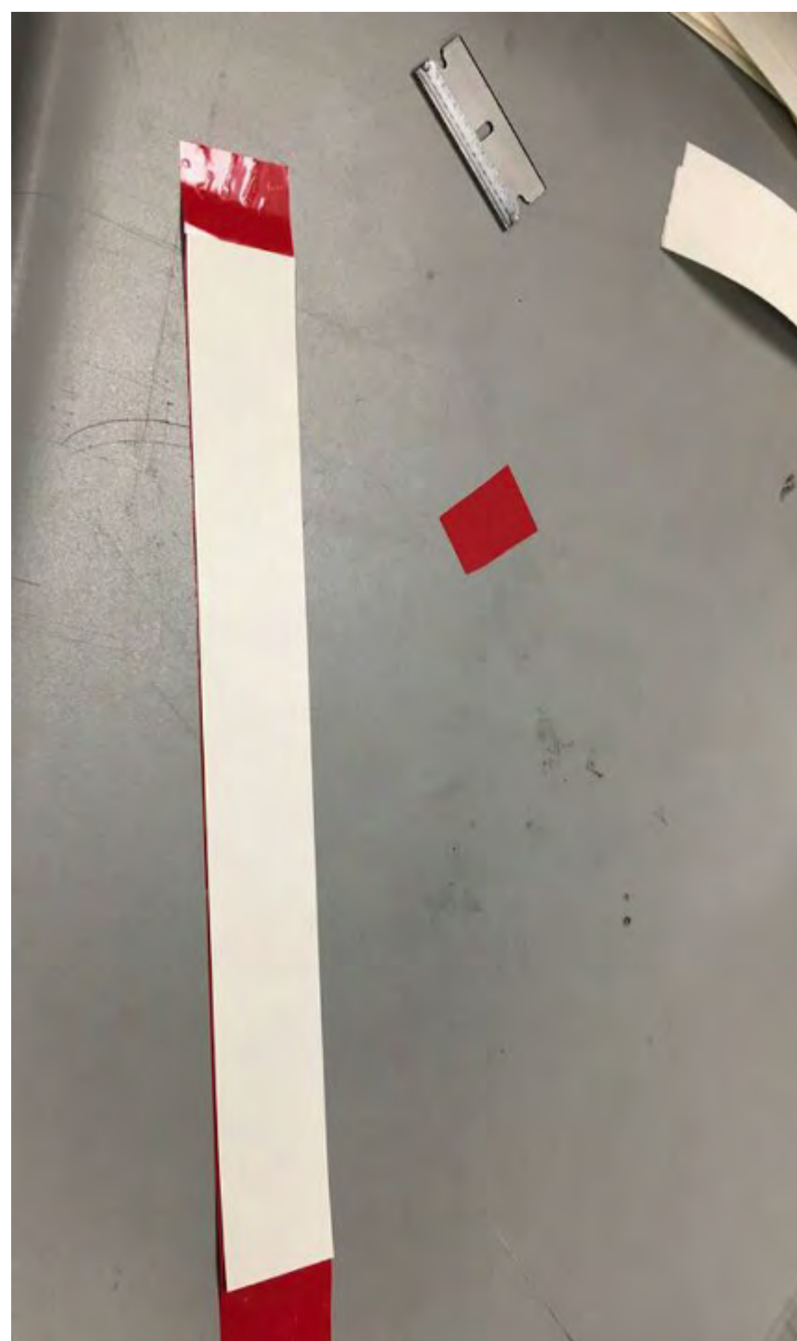
Sample Preparation - cutting samples and applying reinforcements (red tape)
