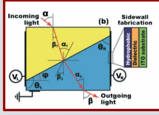
The working principle of the liquid prism is based on the electrowetting phenomenon, which is well described by the Young–Lippmann theory to control the left angle  $\theta_1$  and right angle  $\theta_{R}$  of the prism. The following graphs present the theoretical results which conclude relationship between the prism (apex) angle  $\boldsymbol{\varphi}$  and  $\boldsymbol{\theta}_{I}$  and  $\boldsymbol{\theta}_{R}$  of the prism.
