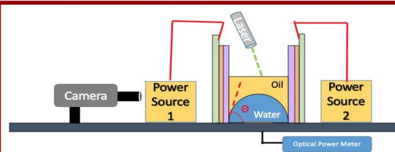
The working principle of the liquid prism is based on the electrowetting phenomenon. When the Voltage is applied on the electrodes, the prism angle shall be changed based on the tension between the wall layers, water and the silicon oil. The more voltage you apply on one side, the more light shall be transmitted through the prism. The prism angle  $\theta$  is around 116°-120° in air. The angle decreases when voltage is applied as shown below.
